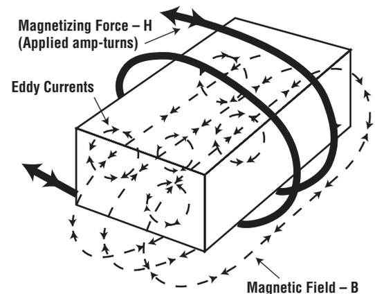
Fig. 10 Energy Loss in form of heat
